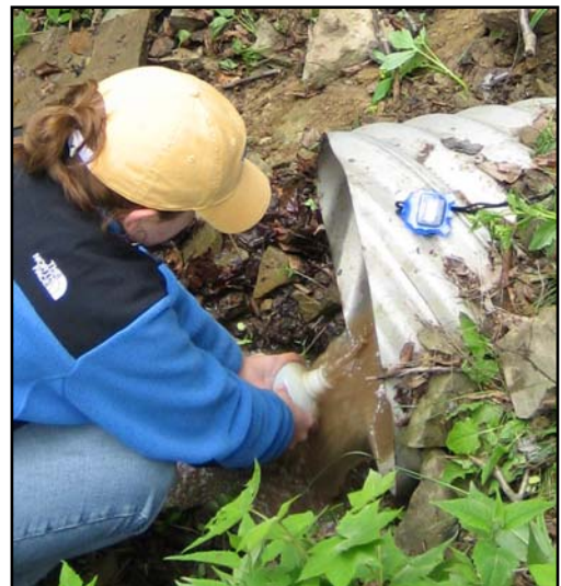
Figure 1.7: A sediment sample is taken at a sample point, in this case a culvert outlet on Lebo Road in Potter County.
