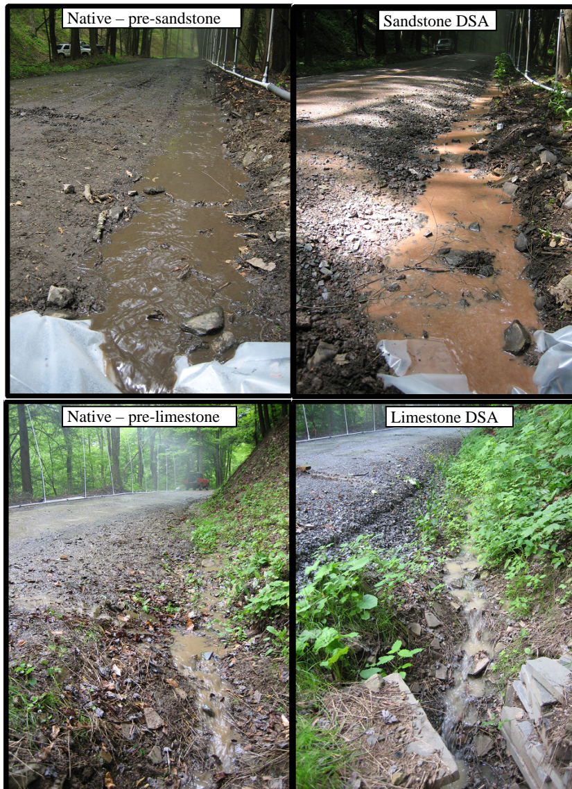
Figure 2.5: Photographs taken during rainfall simulator events for both native and DSA surfaces.
