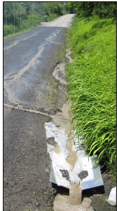
Figure 1.6: This is an example of a rainmaker collection point. Plastic and aluminum sheets are used to concentrate water at sample point.
