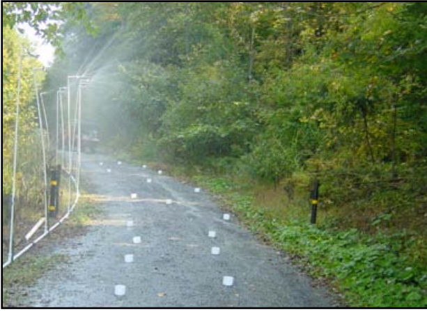
Figure A2: Collection jars for repeatability testing on a test road in Huntingdon County.
