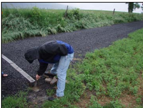
Figure 3.1: A sampling point is cleaned in preparation for a storm event after ESM practice implementation on Goss Lane.
