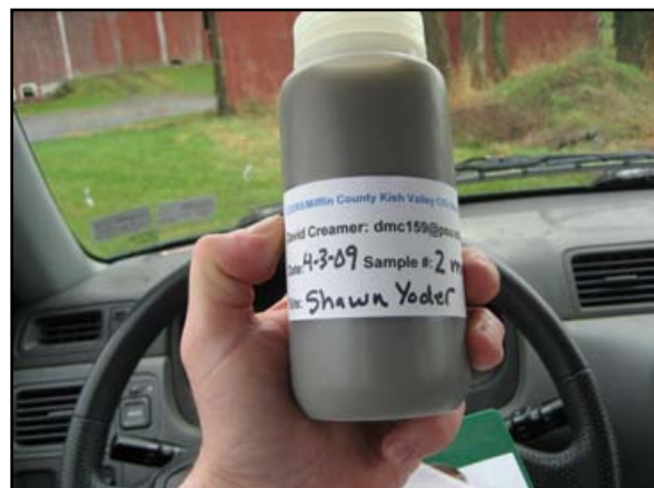
Figure 3.2: A sample bottle of runoff, collected and to be analyzed for sediment and nutrients.
