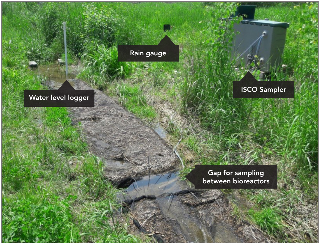
Figure 4. Woodchip bioreactor sock installed in ditch with ISCO sampler housing and rain gauge in the background.
