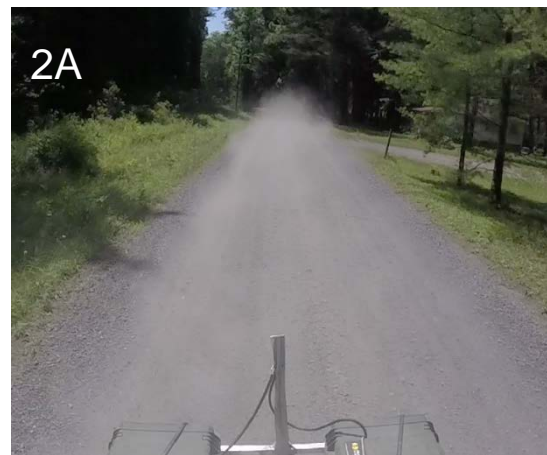
Figure 4. A GoPro camera was mounted on the rear of the vehicle to visually track dust production and canopy openings. The photograph on the left shows the dust production from the DSA 1-2015 section of Laurel Run Road compared to the 2A section on the right.
