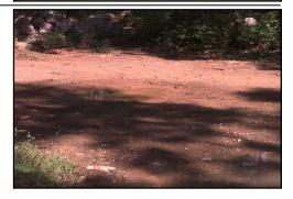
The makeup of the road surface is an important factor in determining the amount of sediment generated form the road area. Studies have shown that sediment generation rates can be 12-25 time higher for native surface roads compared to roads surfaced with quality aggregate.
