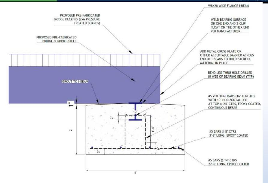
PROPOSED BRIDGE ABUTMENT SECTION (TYP.)
