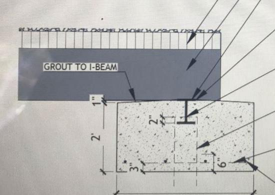
PROPOSED PRE-FABRICATED BRIDGE DECKING (2x6 PRESSURE TREATED BOARDS WITH MEMBRANE & ASPHALT)
