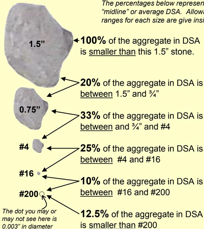
The above illustration shows how the various size components of DSA lock together when compacted to produce the most dense and durable aggregate surface possible. The specification is well graded from large pieces that give support, all the way down to the "fines", rock particles less than 1/300<sup>th</sup> of an inch. This well graded mix including fines allows DSA to achieve a very high density. The box to the left illustrates the actual sizes of a "midline" or average DSA specification.
