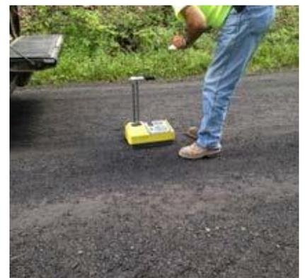
Figure 4: Compaction Testing with Nuclear Density Gauge
