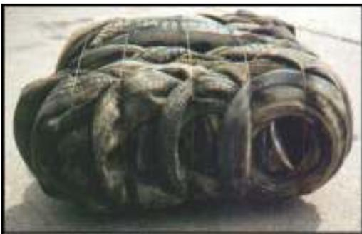
**A tire bale consists of approx. 100 tires, measures 2.5x4.5x5’ and weighs approx. one ton.**
