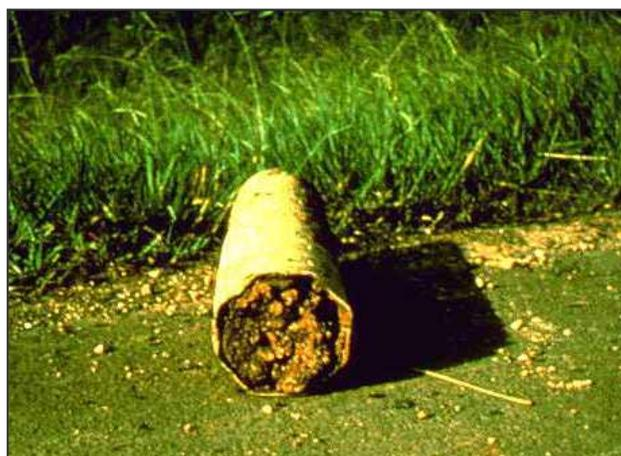
Fabric and outlet protection are important to prevent clogged pipes such as this.
