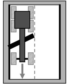
**Figure 2.** Large aggregate that has accumulated on the shoulder is pulled to the center of the road and mixed with fine aggregate particles as it rides up the blade. The blended aggregate is deposited in a windrow in the center of the road. Note the high moisture content of the graded material.
