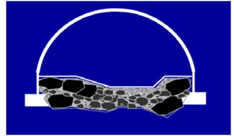
Schematic of a bottomless arch pipe.
