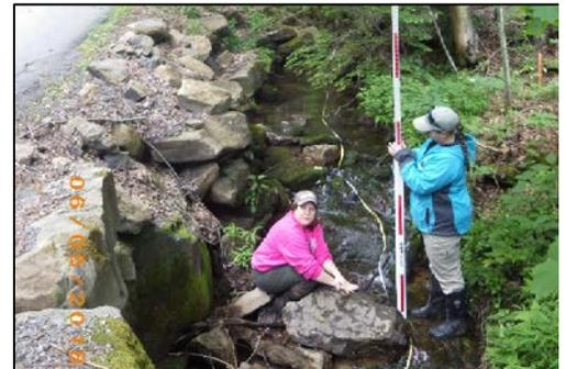
Conducting a longitudinal profile is **essential** to making the best structure selection (ELK).
