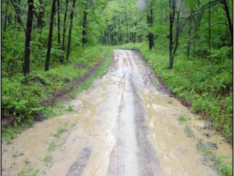
Road shape refers to the cross-sectional profile of the road. Side-slope on a road is vital to insuring water runs perpendicular to the road instead of down the road surface. Crown or cross-slope is a road's first line of defense against erosion. It is very important on steep slopes, since water is more likely to flow down the road.
